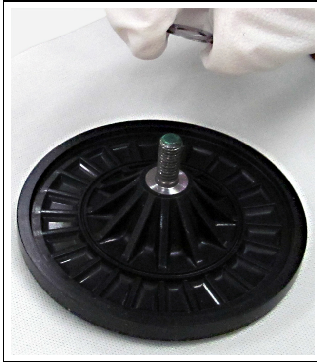
Figure 7-11 Placing original spacers on new diaphragm
